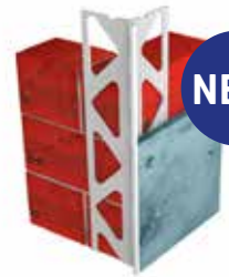
341000 M PVC angle bead white 10 mm render dimensions 40 × 40 mm
