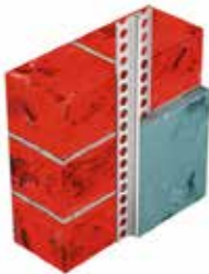
200600 depth gauge profile PVC 10 mm render dimensions 36 × 10 mm
