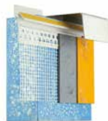
640000 Attika PVC end profile with mesh 5 mm render
