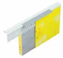
156600 end profile PVC with pull-out cover strip dimensions 30 × 12.5 mm
